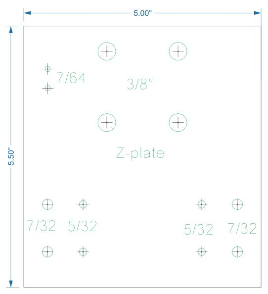
Tap four 5/32 holes with 10-32 Tap Tap the two 7/64 holes with 6-32 Ream 3/8" holes with 1/2" bit Stock is 5" wide by 5.5" tall
