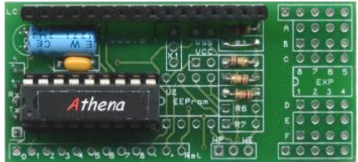
Figure 4: Populated PCB with female header.
