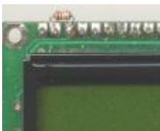
Figure 3: Small contrast resistor connected to LCD.
